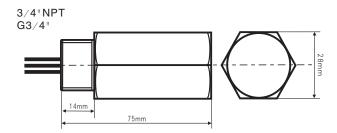
Note: Wire size 26/0.254 (1.32mm<sup>2</sup>, 16AWG), length 150mm.
