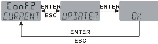
Set current output, enter menu "Conf.2 CURRENT", after receiving request of "UPDATE?", press Key ENTER, displays"OK", parameter setting successfully. Instrument is set to this state when leaving the factory.
