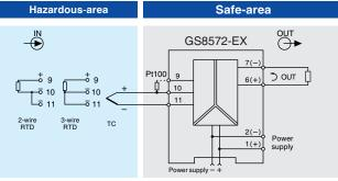
Note:2-wire connection can not erase lead resistance, error increases.
