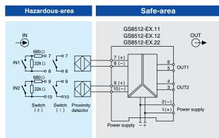
Note: GS8512-EX.11,only contains input1, output1; GS8512-EX.12 the input part only contains input 1.
